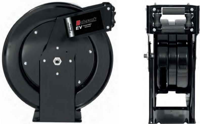
The Extended Volume, EV Series hose reels are designed for high volume heavy-duty applications where large hose diameters are required for increased flow. The EV reels will accommodate up to 50' of 3/4" ID hose or 65' of 1/2" ID hose. Perfect for heavy-duty fleet, construction, mining and industrial applications. All EV series reels include hose, hose stop and a 2.5' connecting hose.
