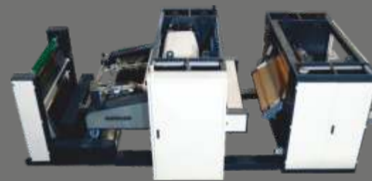
Compactor Machine For Tube Knitted Fabrics
