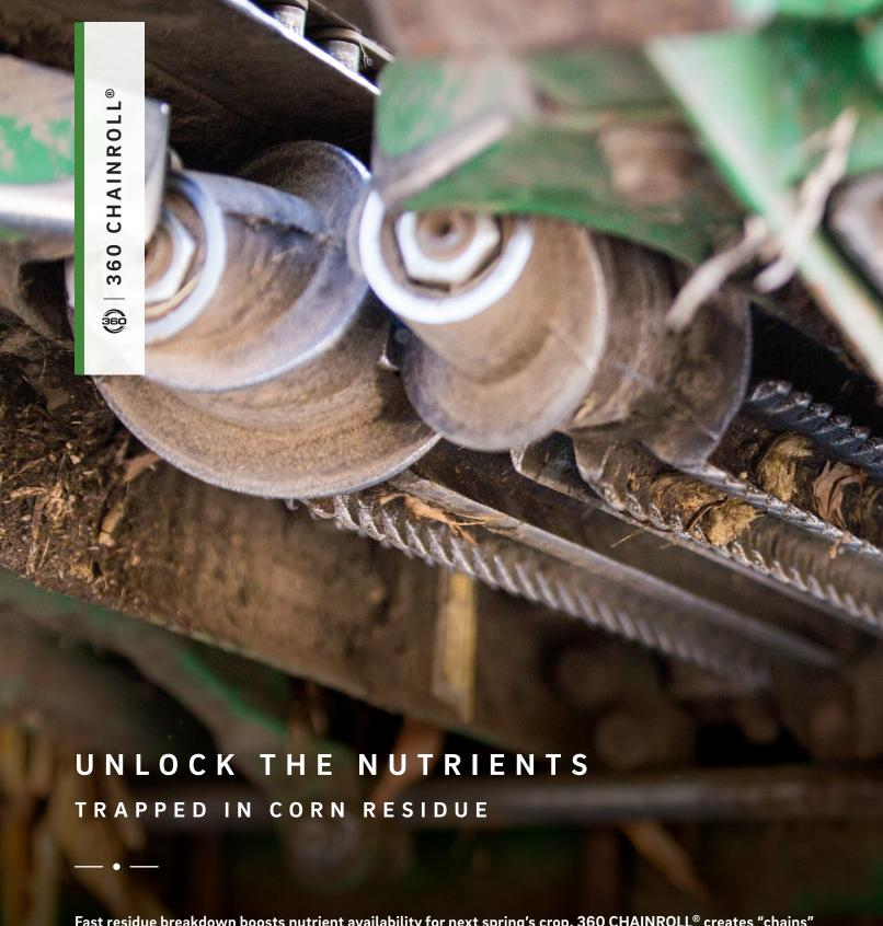
Fast residue breakdown boosts nutrient availability for next spring's crop. 360 CHAINROLL® creates "chains" of seven-inch stalks - ideal for rapid breakdown. Plus, they're the perfect length for row cleaners to remove from the seed trench.
