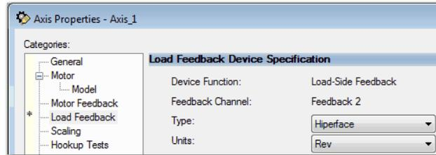
Unlike the Motor Feedback category, you must explicitly enter load feedback-device information on the Load Feedback category, including the Feedback Type. This entry is required because the Load Feedback device is not built into the motor.
