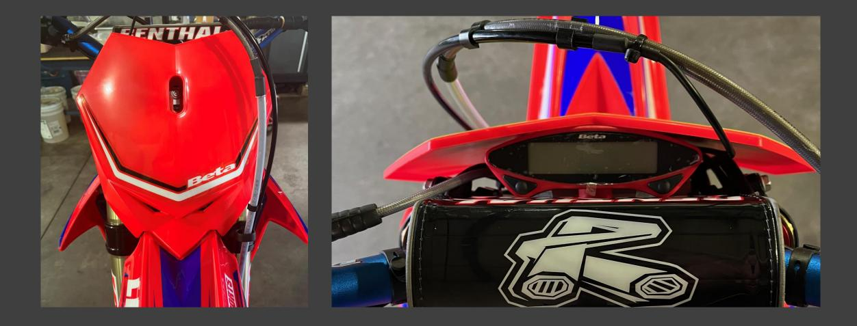
Reinstall head light mask/racing plate
