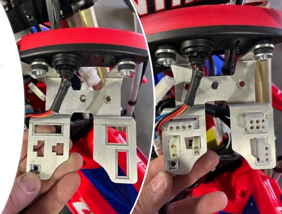
13. Mount new bracket using the included hardware and apply a small amount of blue Loctite, torque to 6NM.
