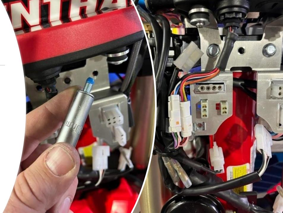
14. Reinstall bolt for wire harness strap, take some time to zip tie wire harness well to avoid any rubbing or chaffing.
