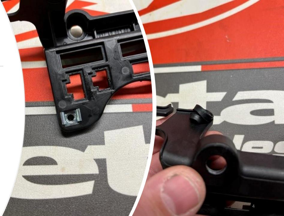
9. Install pinch nut into new meter bracket as shown.
