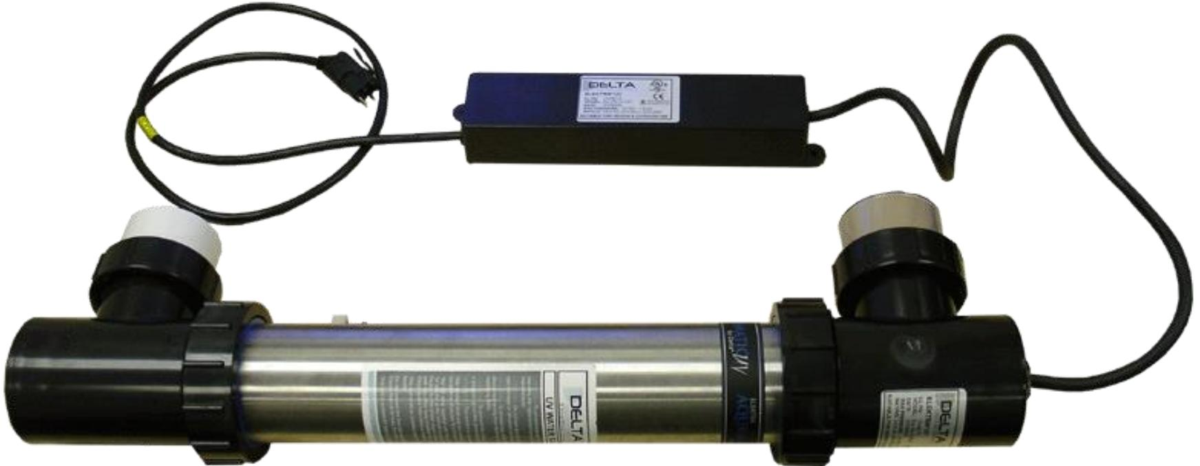
The Delta UV will be used as an example. Essentially spa water flows through the stainless tube housing which holds a light bulb which radiates passing germs and makes them incapable of reproducing.
