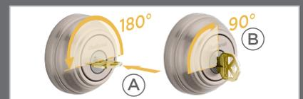
**3** (A) Fully insert new key & rotate 180°.
