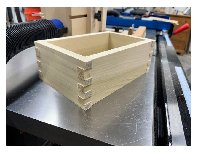
The most commonly used box-joint jig cannot cut patterns like this. The Ruud Complement Jig provides one way to make this joint. After first cutting one-half of the joint on one side, the other half is cut from the first, using the first as a template.
