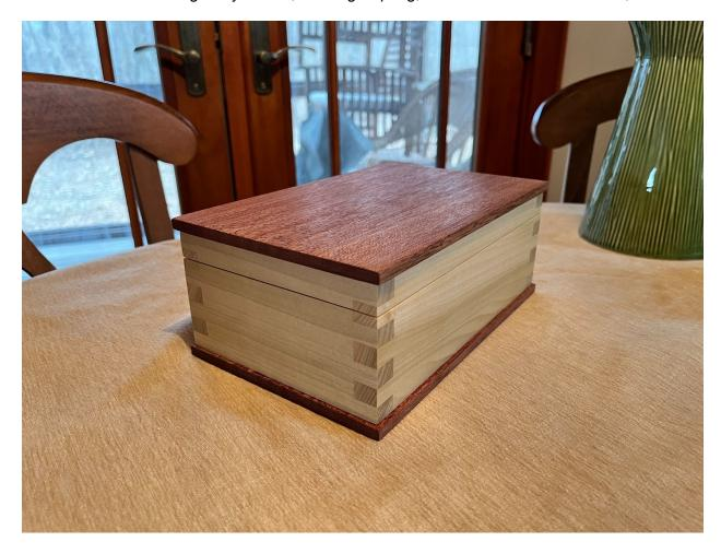
This is an example of a box with sides connected by box joints. While the spacing between sockets appears to be consistent, to make this box (with it's cut-off lid) one of the pins has to be extra wide to account for the saw blade kerf. Here is a picture of the box sides before glue up:
