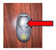
2. Press and hold the red button for about three (3) seconds until the LED light turns red.
