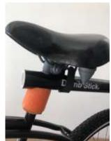
THE ATTACHED ANTI – SWAY STRAP ELEVATES THE DUMB STICK AND ALSO PREVENTS THE DUMB STICK FROM PIVOTING SIDE TO SIDE.
