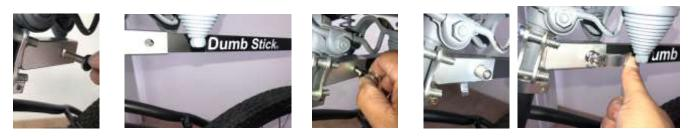
Step 8 Attach the silver clip to the eye hook at the end of the Dumb Stick Bar.
