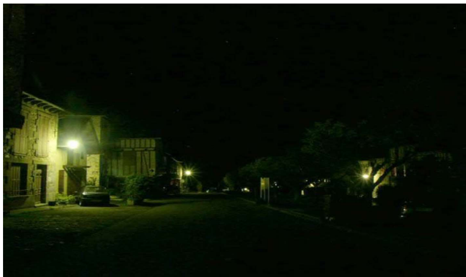
Figure 2: Village of Najac/FR before the installation of new LED streetlights. This photograph shows the old mercury-vapor lamps which produce white light with a bluish-green hue and a very low CRI. Such light is harsh and uncomplimentary to the surrounding architecture and various building materials and it is also unflattering to human skin tone. © Wonderfulight
