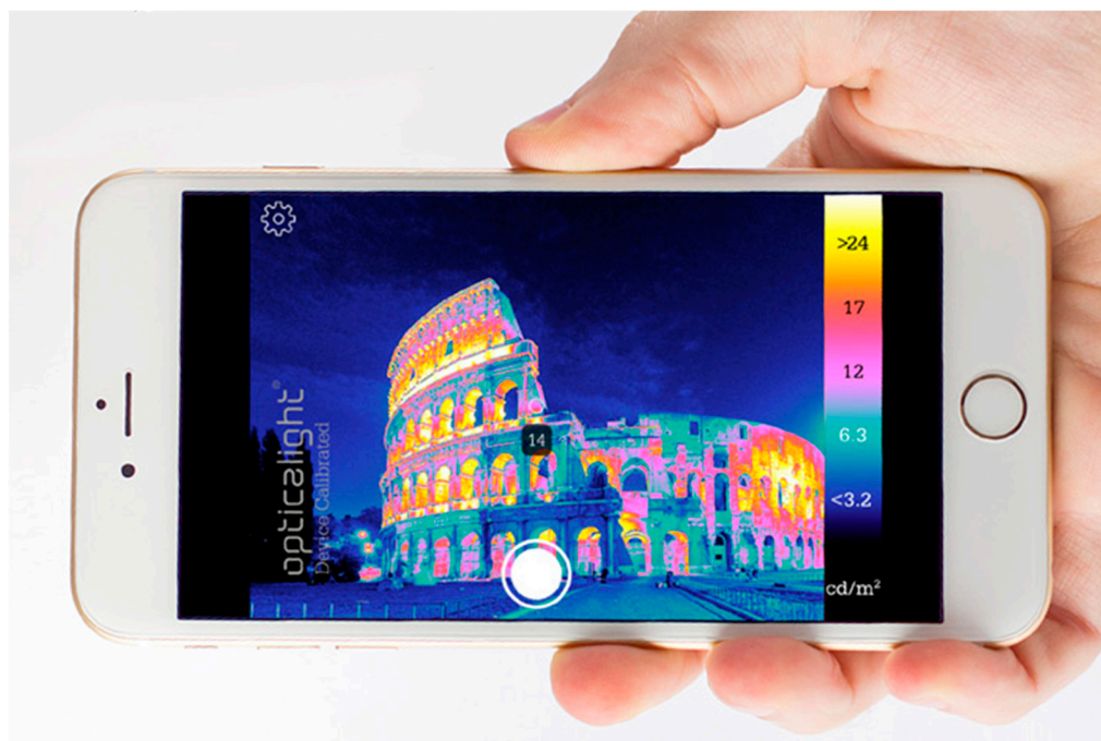
Figure 5. An example of the results from a typical outdoor luminance measurement in \text{cd/m}^2 taken by a video luminance meter mobile phone application with a false color image function for easy evaluation. False color assigns different colors to areas of different luminance exposure in the image. Source: Opticalight's figure.
