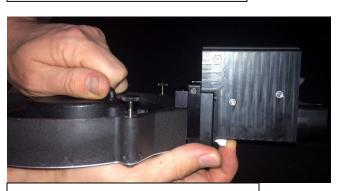
**3.** Put Mag-Top on and press down activator while holding middle rotor and let it slowly unwind. Be careful, there can be a lot of tension in the drum.
