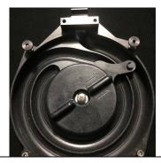
1. Rotate rotor to this exact position and remove backplate. This is the **Start** position.
