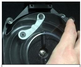
2. Remove back plate by loosening the thumbscrews, rotating back plate to the left, and pull up and off.
