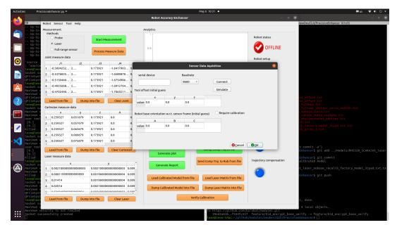
Clicking the sensor menu will pop up a new GUI window. On the top of GUI, users need to enter the serial device name (e.g. "/dev/ttyACM0"), choose the correct Baud Rate, and then click "connect". If communication is okay, the "connect" button will turn green.
