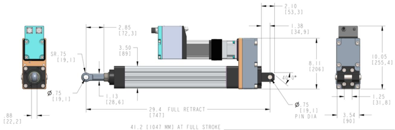
The EDGE actuators are designed for web and strip guiding.
