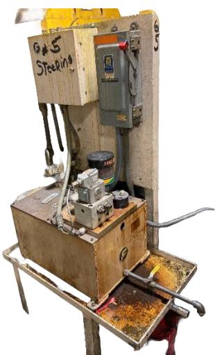
Replace Maxcess/Fife power units. These units have been obsolete for over 10+ years. Spare parts are also obsolete.
