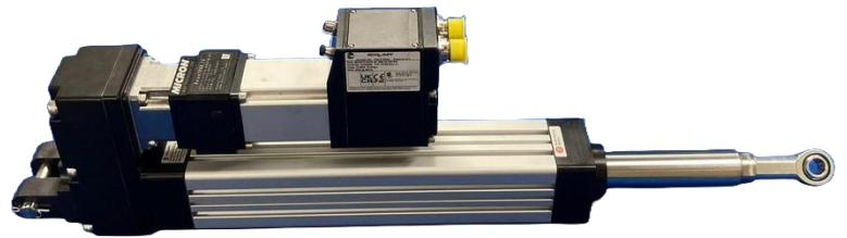
Upgrade your obsolete, brushed DC motor which is controlled by a remote motor drive. **High thrust actuators, rated in 2,000, 4,000, and 6,500 ft-lbs. of thrust utilize DC brushed motors.** The brushes require maintenance. The manufacturers of the motors are gradually obsoleting the motors and therefore the actuators will also become obsolete. The linear thrust is produced by a **ball-screw actuator** which under-performs as the thrust increases.
