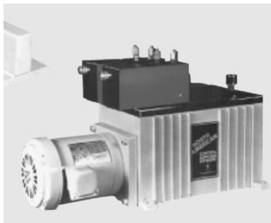
Replace pneumo-hydraulic power units. These units have been obsolete for over 10+ years. Spare parts are also obsolete.
