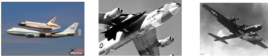
Figure 5 Methods of One Aircraft Carrying Another
