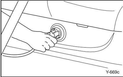
3. With the charger properly connected and grounded (see charger's owner's manual), insert the DC output into the golf car receptacle.
