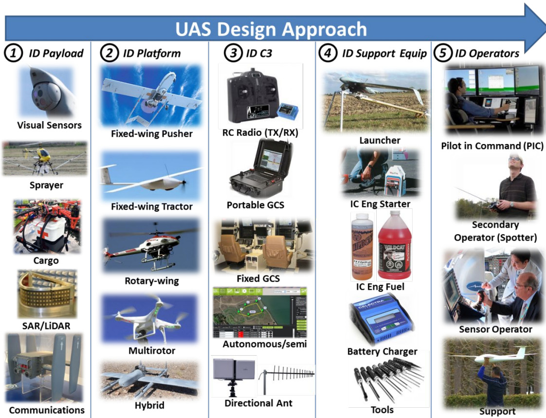
Figure 2. UAS design approach with major element options identified.
