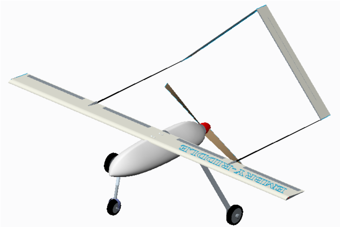
Figure 8. Fixed-wing pusher propeller design.
