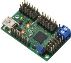
High-fidelity/onboard sensing option that can be connected to a communication device (i.e., telemetry radio) using a serial interface to transmit analog and digital sensor data to a PC.
