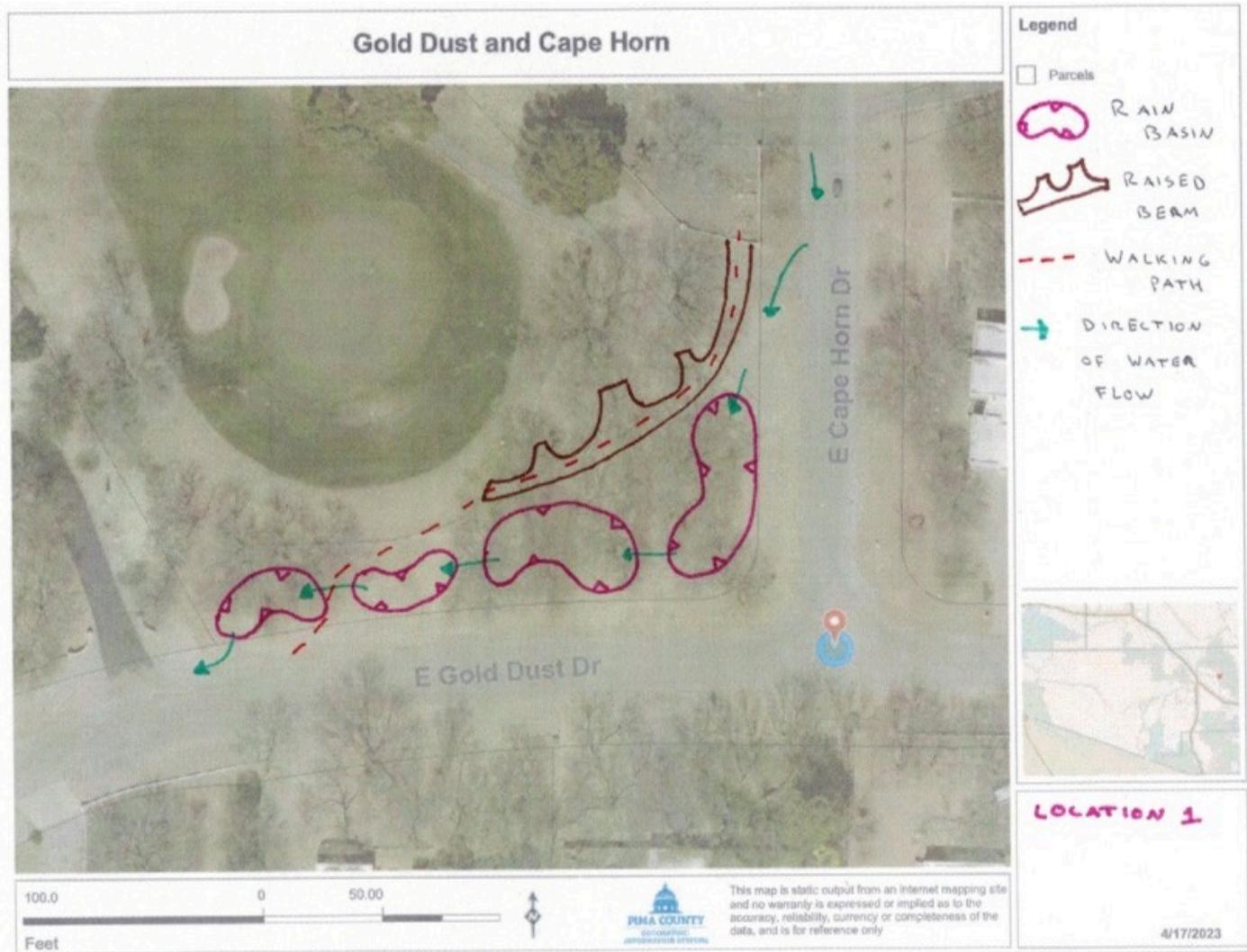
Figure 5. Proposed stormwater harvesting project for location 1.
