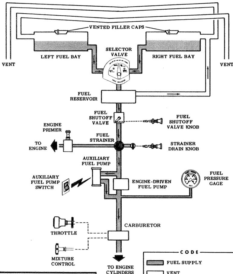
TO ENSURE DESIRED FUEL CAPACITY WHEN REFUELING, PLACE THE FUEL SELECTOR VALVE IN EITHER LEFT OR RIGHT POSITION TO PREVENT CROSS-FEEDING.
