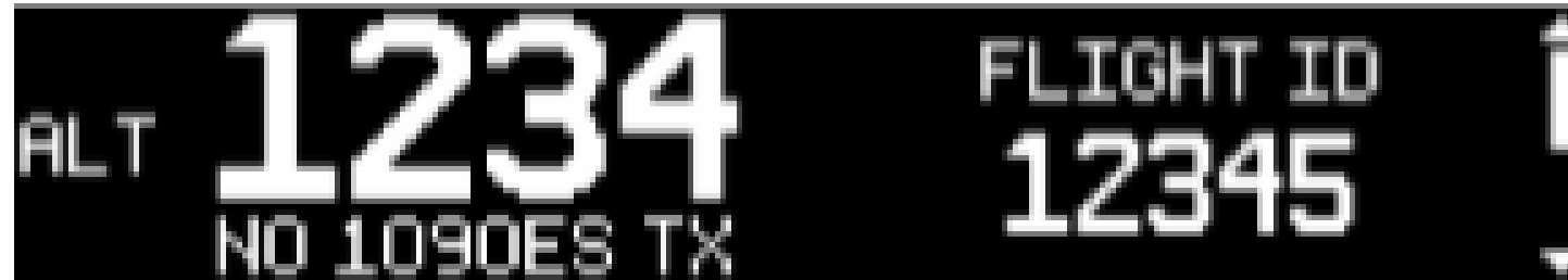
Figure 7-1 ADS-B 1090 Failed Screen
