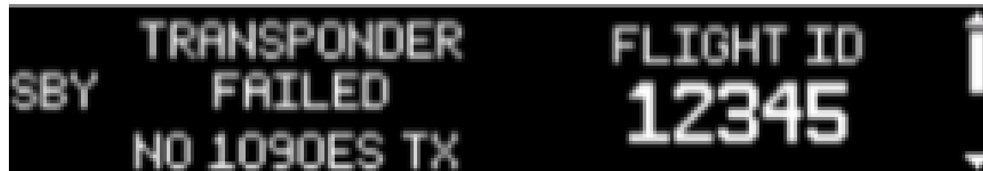
Figure 7-2 ADS-B 1090 and Transponder Failed Screen
