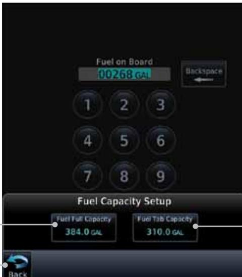
Figure 1-15 Fuel Capacity Setup Page
