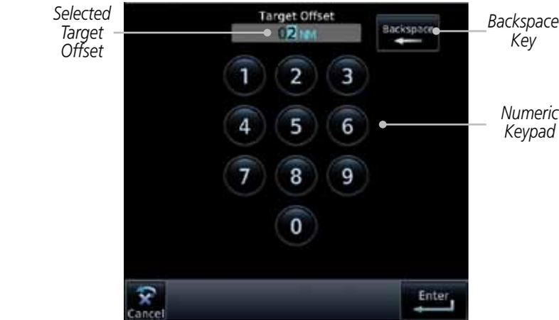
Figure 15-8 Select VCALC Target Offset
