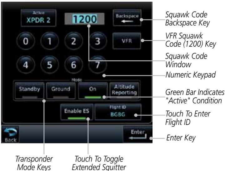
**Figure 2-12 Transponder Control Panel With Extended Squitter Capability**
