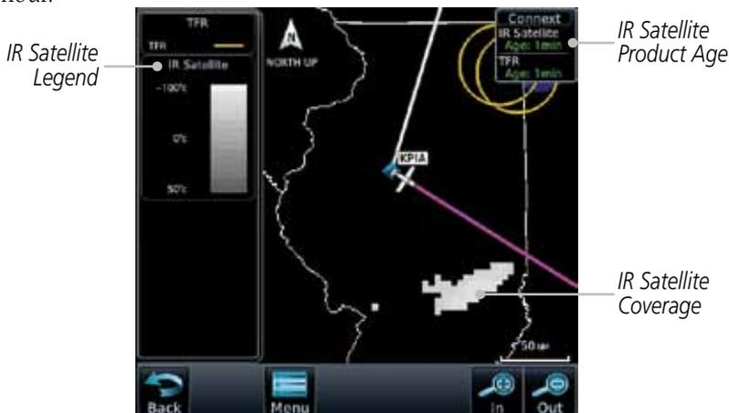
Figure 12-80 ConnexT Infrared Satellite Data Map Display and Legend
