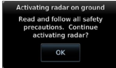
Figure 12-57 Caution for Radar Activation Confirmation
