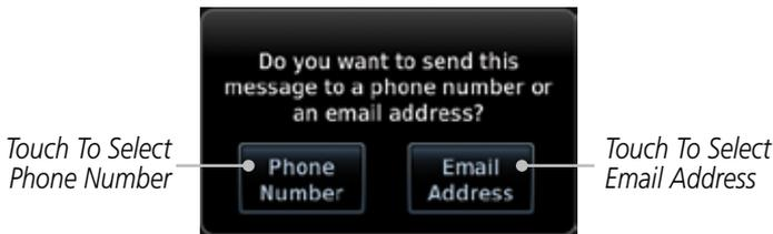
**Figure 14-24 Select Destination for the SMS Text Message**
