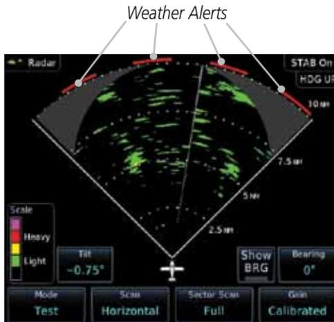
**Figure 12-66 Weather Alert Display**
