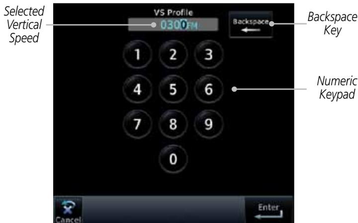
**Figure 15-7 Select VCALC Vertical Speed**
