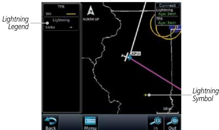
Figure 12-79 ConnexT Data Link Lightning and Legend
