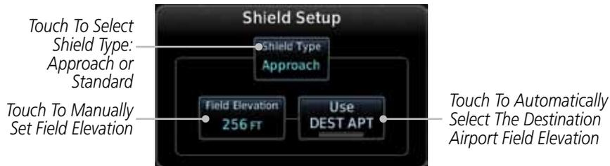
**Figure 10-28 TCAD 9900B Shield Setup for Approach**
