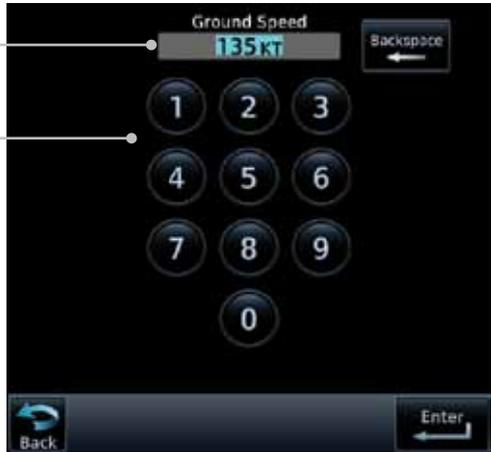
Figure 15-18 Selecting Expected Average Ground Speed
