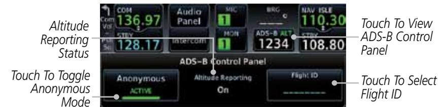
Figure 2-10 ADS-B Control Panel
