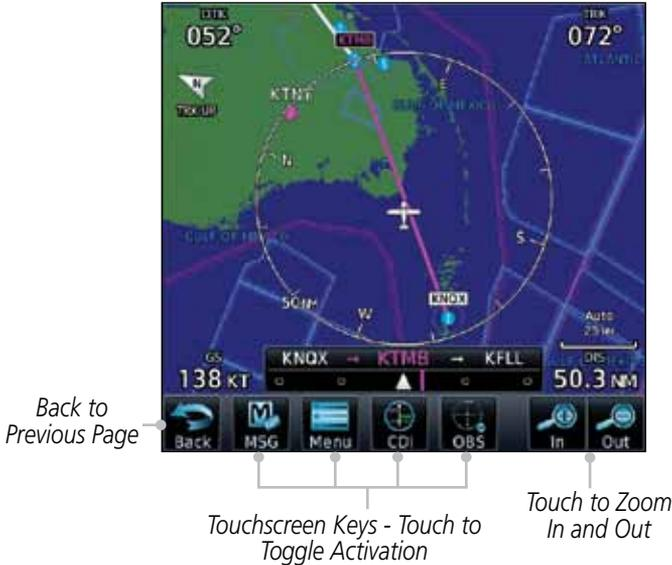
Figure 1-18 On-Screen Keys and Active Display Areas
