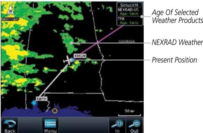
Figure 12-8 SiriusXM NEXRAD Weather
