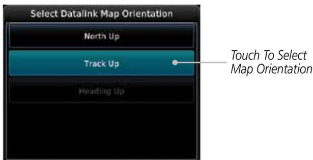
**Figure 12-73 Connex Weather Map Orientation**
