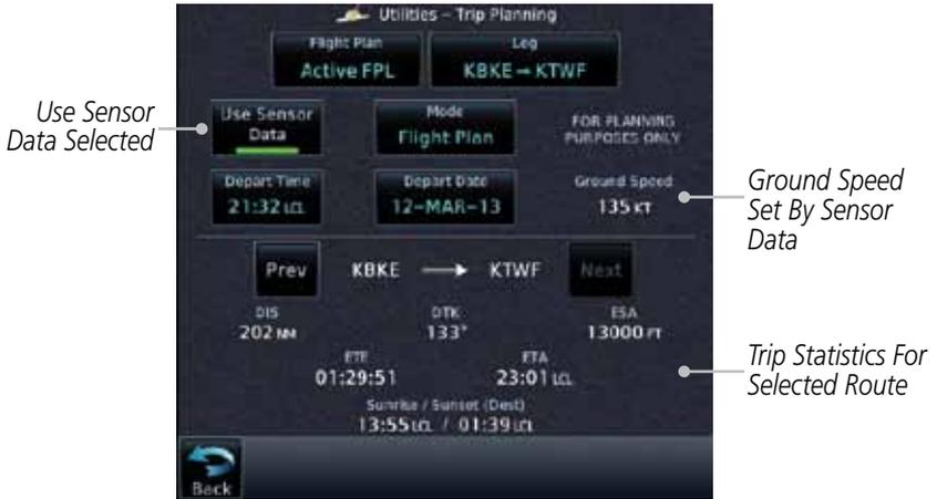
Figure 15-25 Utility Trip Planning Page Computed Data View (Flight Plan Mode) - Use Sensor Data Selected
