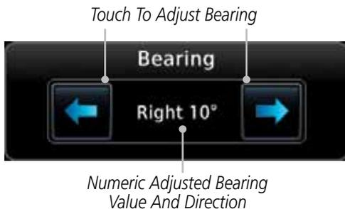
**Figure 12-60 Bearing Line Adjustment**
