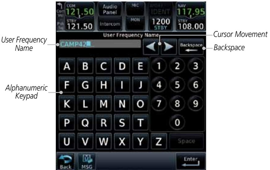
Figure 3-16 Select a Name for the New User Frequency
