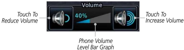
**Figure 14-20 Select Soft Keys for Phone Volume Adjustment**
