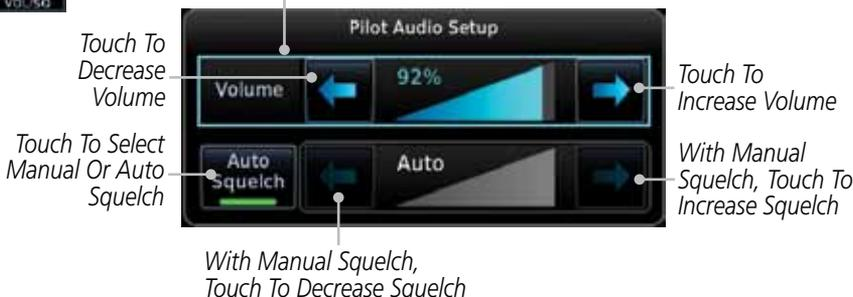
**Figure 2-22 Pilot Audio Setup**
