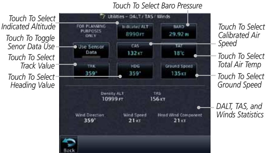
**Figure 15-37 Utility DALT/TAS/Winds Page Using Manually Entered Data**
