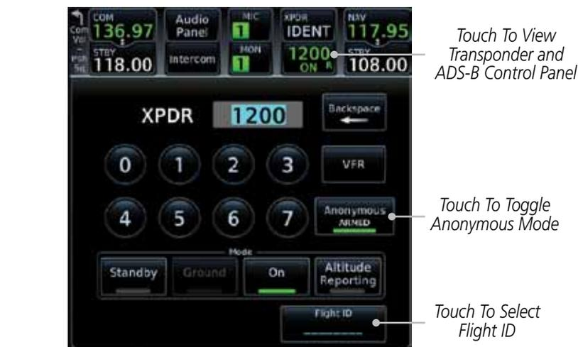
Figure 2-11 ADS-B/Transponder Control Panel
