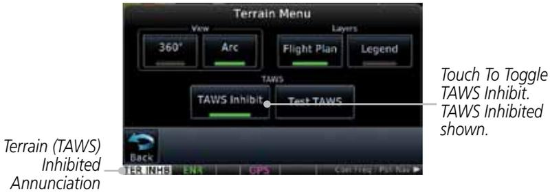
Figure 11-14 TAWS Alerting Disabled (TAWS Inhibited) Annunciation
