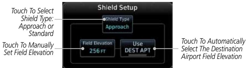
Figure 10-34 TCAD 9900BX Shield Setup for Approach
