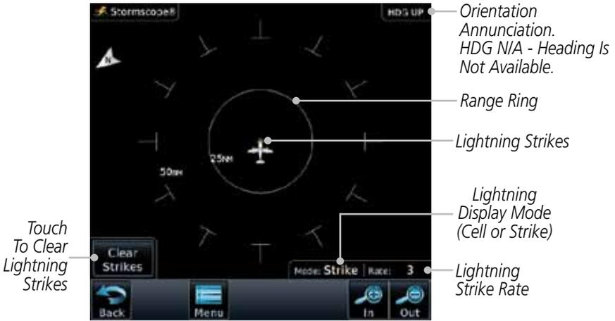
Figure 12-40 StormScope Display (360° Display View Shown)
