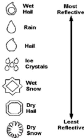
Figure 12-46 Precipitation Type and Reflectivity
