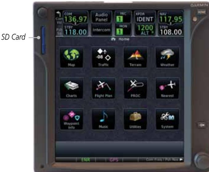
**Figure 19-1 SD Card Database Location**
