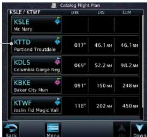
**Figure 4-11 New Waypoint Is Inserted Before the Selected Waypoint**
