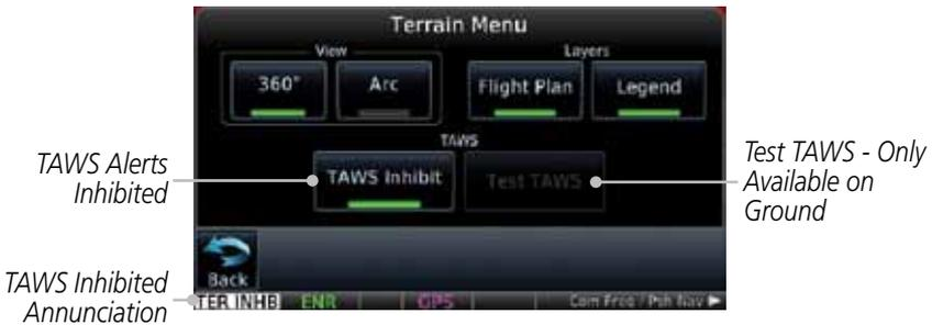
Figure 11-9 TAWS Alerts Inhibited Selected
