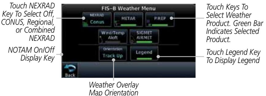
Figure 12-91 FIS-B Weather Data Link Menu
