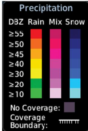
**Figure 12-78 Connex PRECIP Weather Map Display and Legend**
