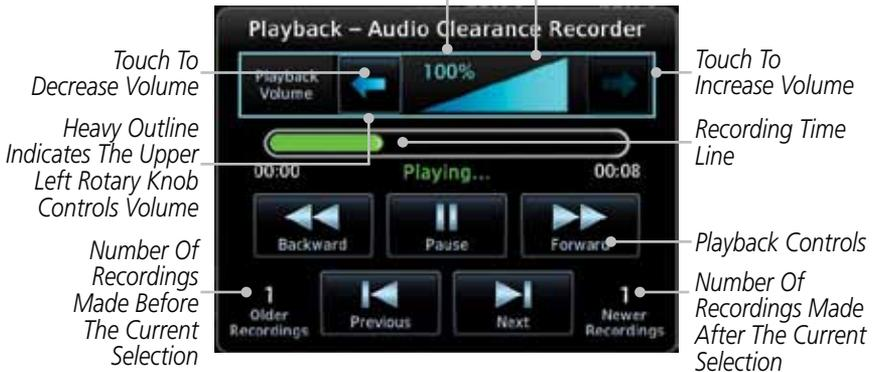
**Figure 2-19 Audio Panel Playback Controls**
