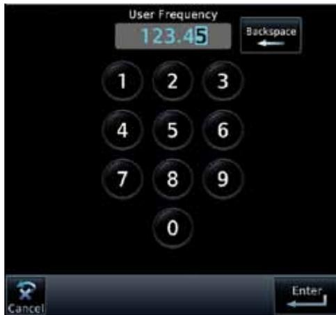
Figure 3-17 Select a Frequency Value for the New User Frequency
