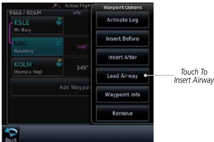
Figure 4-18 Select Load Airway from the Waypoint Options
