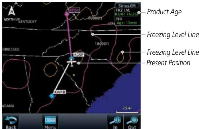
Figure 12-22 Freezing Level
