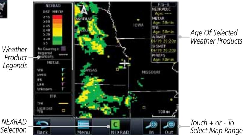
Figure 12-90 FIS-B Weather Page (NEXRAD Key Shown)
