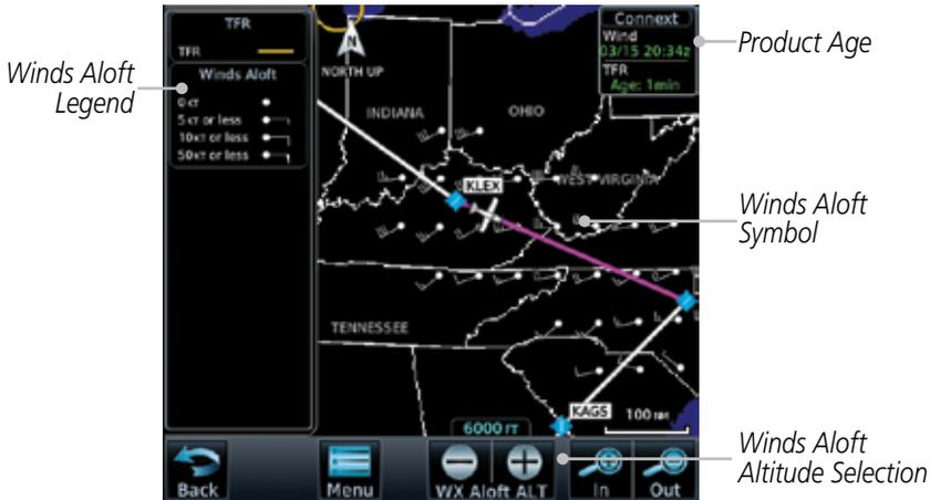
Figure 12-84 Connex Weather - Winds Aloft
