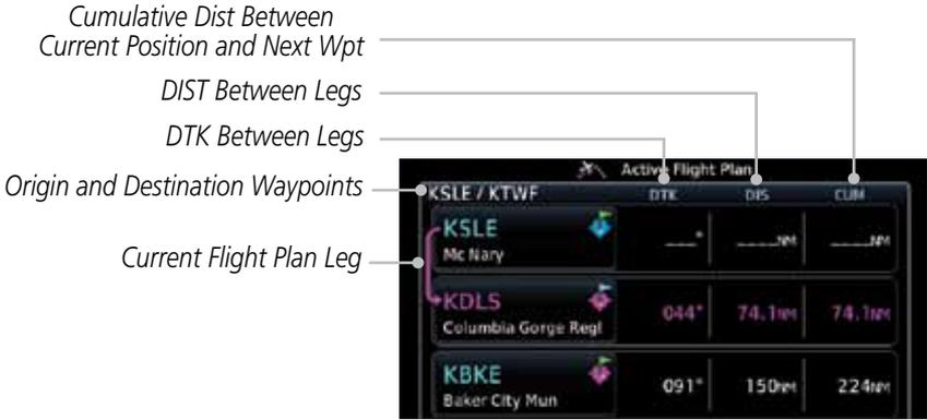
Figure 4-32 Flight Plan Data Fields
