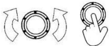
**Figure 3: Knob rotation and pushbutton actions.**
