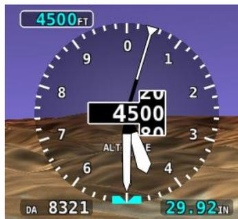
Figure 78: New Instrument Altitude Gauge
