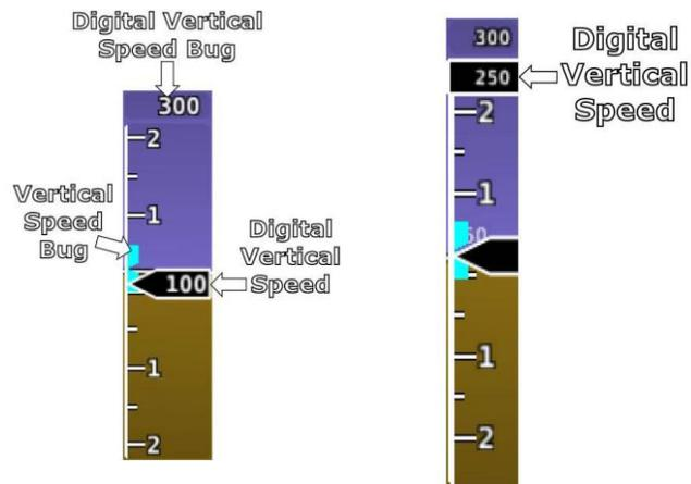
Figure 39: Vertical Speed Indicator example
