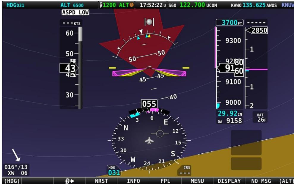
Figure 74: Extreme Pitch warning indicator arrows
