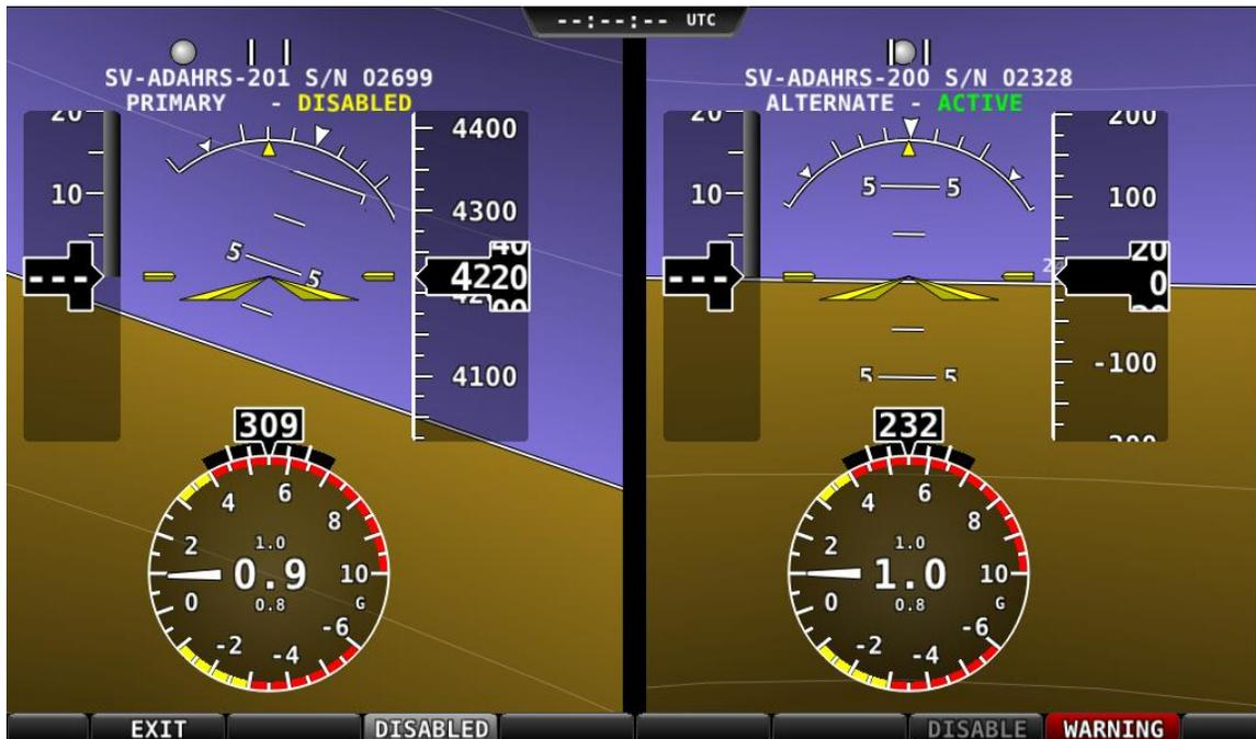
Figure 89: ADAHRS cross-check comparison (one ADAHRS disabled).
