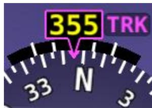
**Figure 41: GPS Track substitute for Magnetic Heading indicator**
