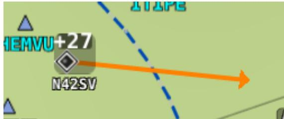
Figure 122: Displaying tail number on Traffic targets.
