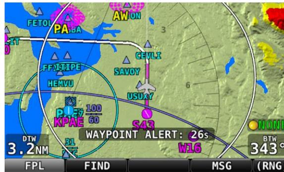
Figure 158: Flight Plan alert messages
