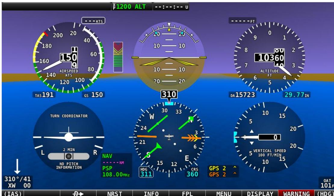
Figure 76: Six Pack PFD presentation, Synthetic Vision enabled.
