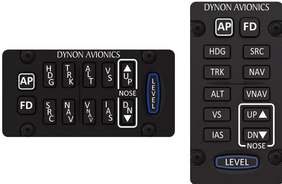
Figure 238: SkyView Autopilot Control Panel
