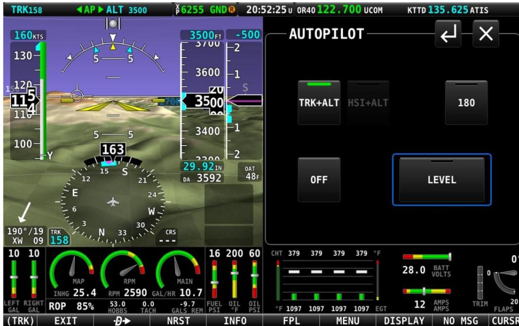
Figure 223: TRK+ALT mode is engaged.
