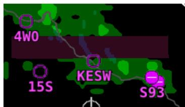
Figure 174: Missing NEXRAD data blocks.
