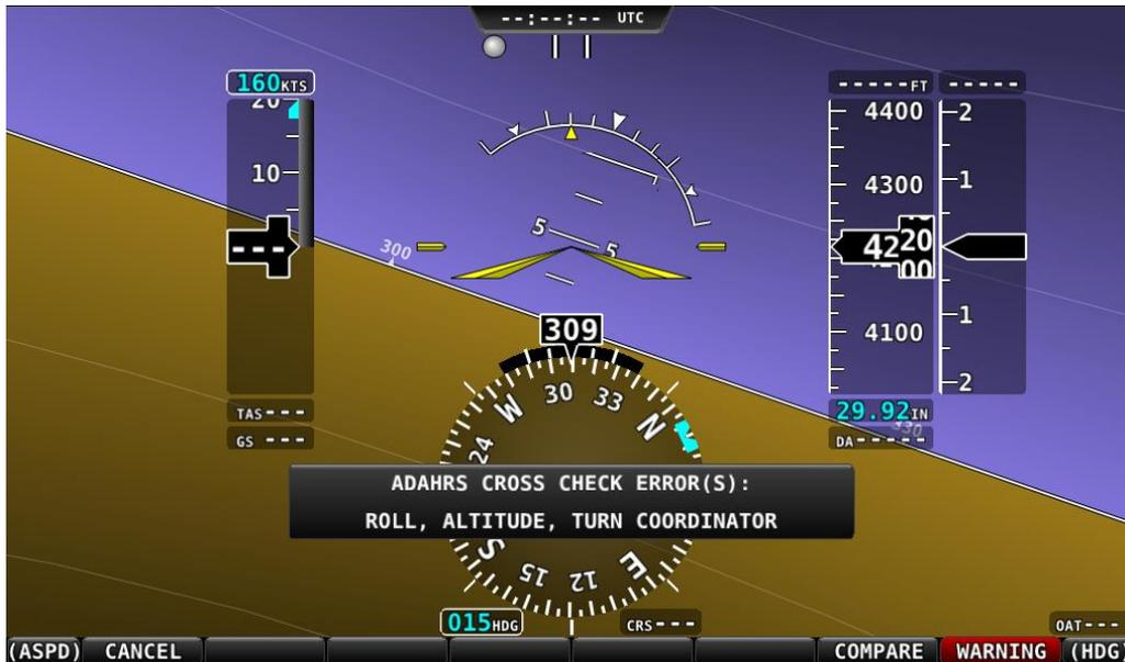
Figure 87: ADAHRS cross-checking disagreement.
