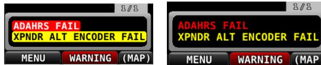
**Figure 251: Unacknowledged (left) and Acknowledged (right) alerts**
