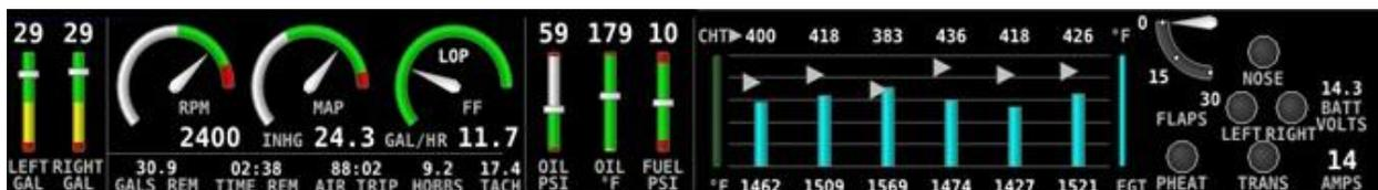
Figure 194: Example of an ENGINE BOTTOM BAND Page layout for single-engine monitoring.
