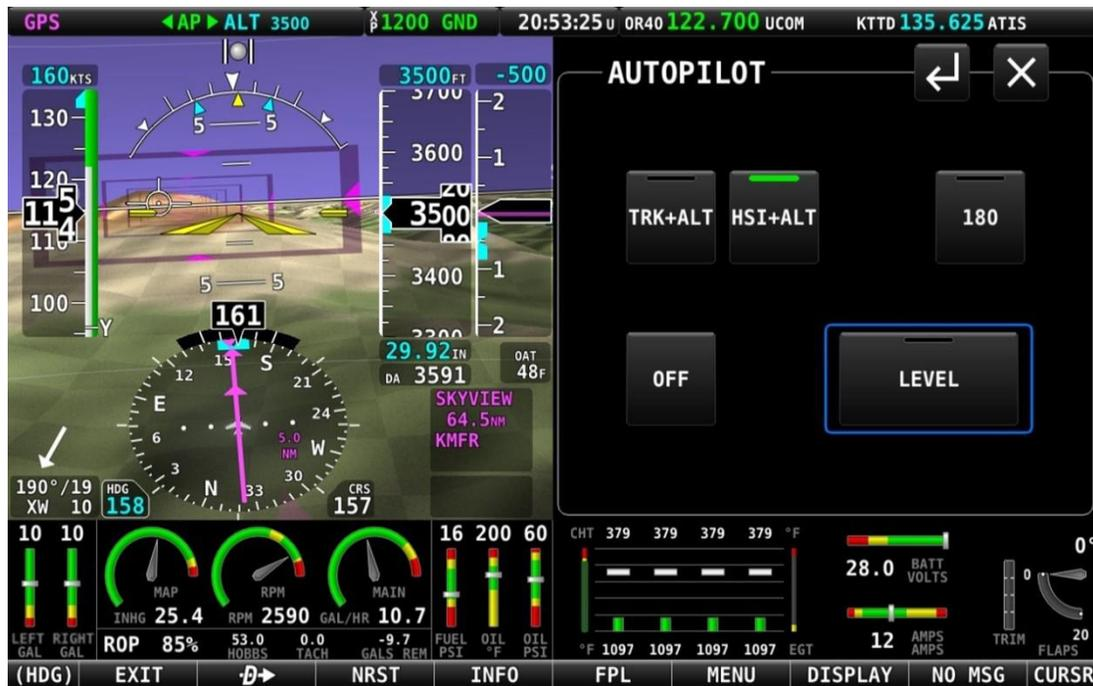
Figure 224: HSI+ALT Mode is engaged.
