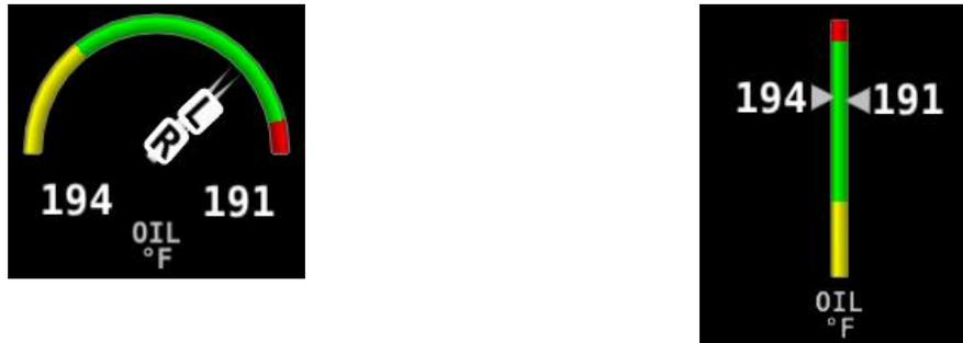
Figure 197: Examples of combined Oil Temperature widgets.
