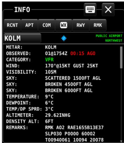
Figure 184: METAR – decoded
