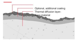
1 Thermal diffusion layer:Micro alloy of zinc and base material
