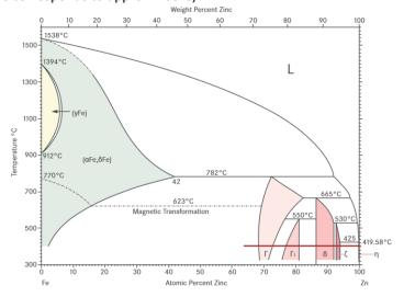
According to the Fe-Zn phase diagram, the sequence of intermetallic phases (microalloys) of the steel/iron in the direction of the surface is as follows:  $\alpha$  (ferrite solid solution of the steel/iron),  $\Gamma$ ,  $\Gamma_1$ ,  $\delta$ ,  $\zeta$ ,  $\eta$  (zinc solid solution); valid between 300 - 400°C. Using the REM line scan, the local composition of the layer structure can be analyzed.
