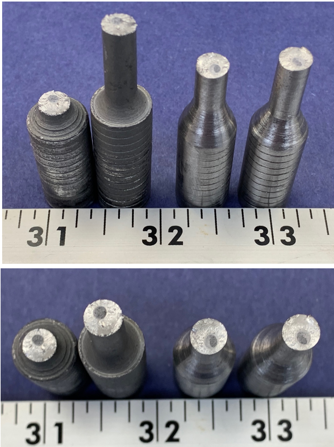
Figure 2: Photograph of the (left) TDZ and (right) bare bolt fatigue testing specimen after fracturing to observe the crack propagation. The dark gray area is the final fracture surface that occurred during the crack opening process.
