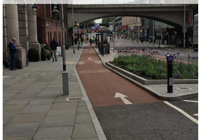
Figure 9.4: Cycle lane to cycle track transition
