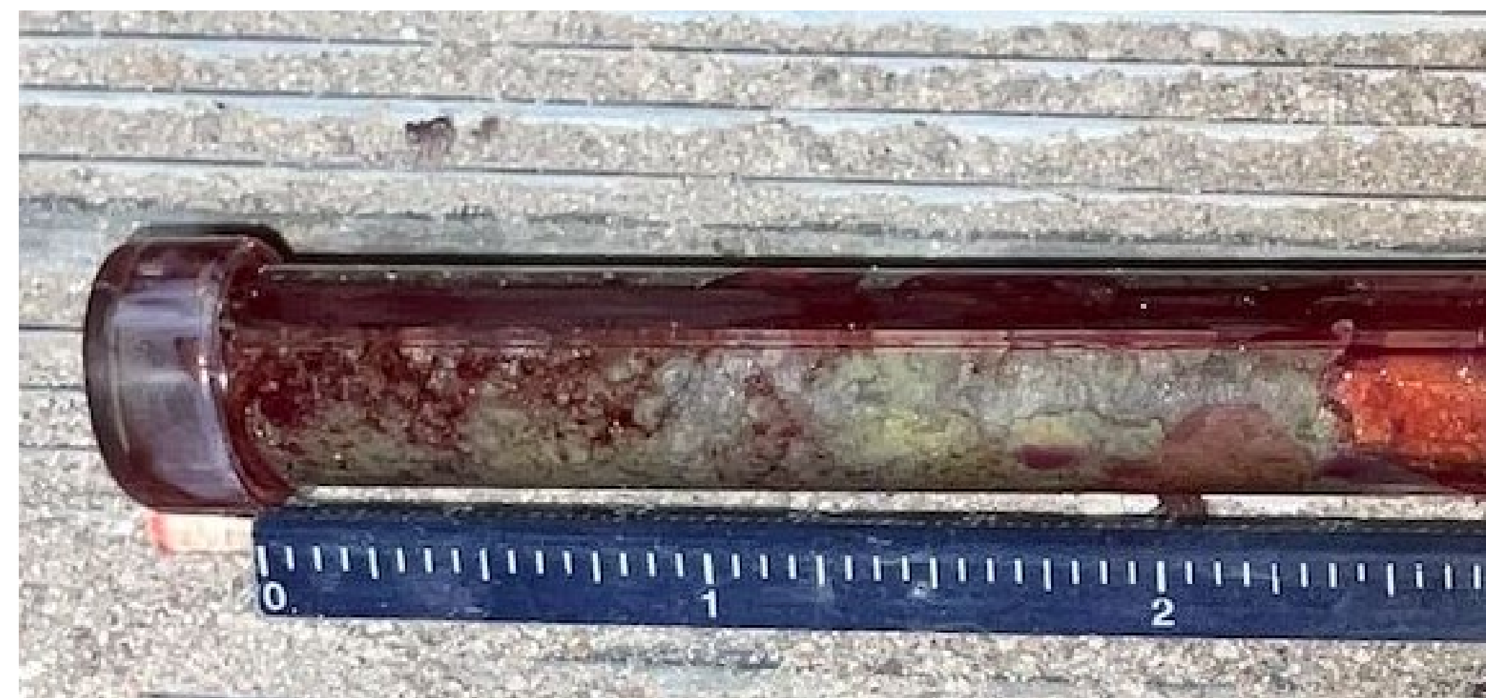
On-site carbonation testing
