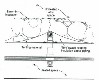
FIGURE A.5.4.2(f) Insulation Recommendations — Arrangement 6.
