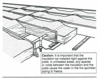
FIGURE A.5.4.2(a) Insulation Recommendations — Arrangement 1.
