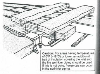
FIGURE A.5.4.2(b) Insulation Recommendations — Arrangement 2.
