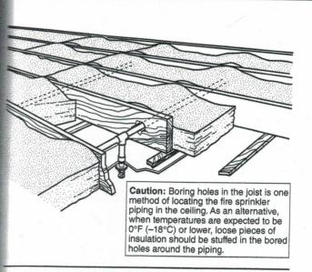
FIGURE A.5.4.2(c) Insulation Recommendations — Arrangement 3.
