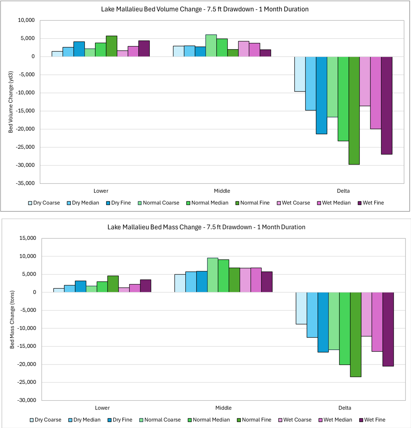
Figure 17. Changes in bed volume (top) and mass (bottom) for segments through the Lake Mallalieu impoundment during the drawdown period of September to October for the 7.5 drawdown.
