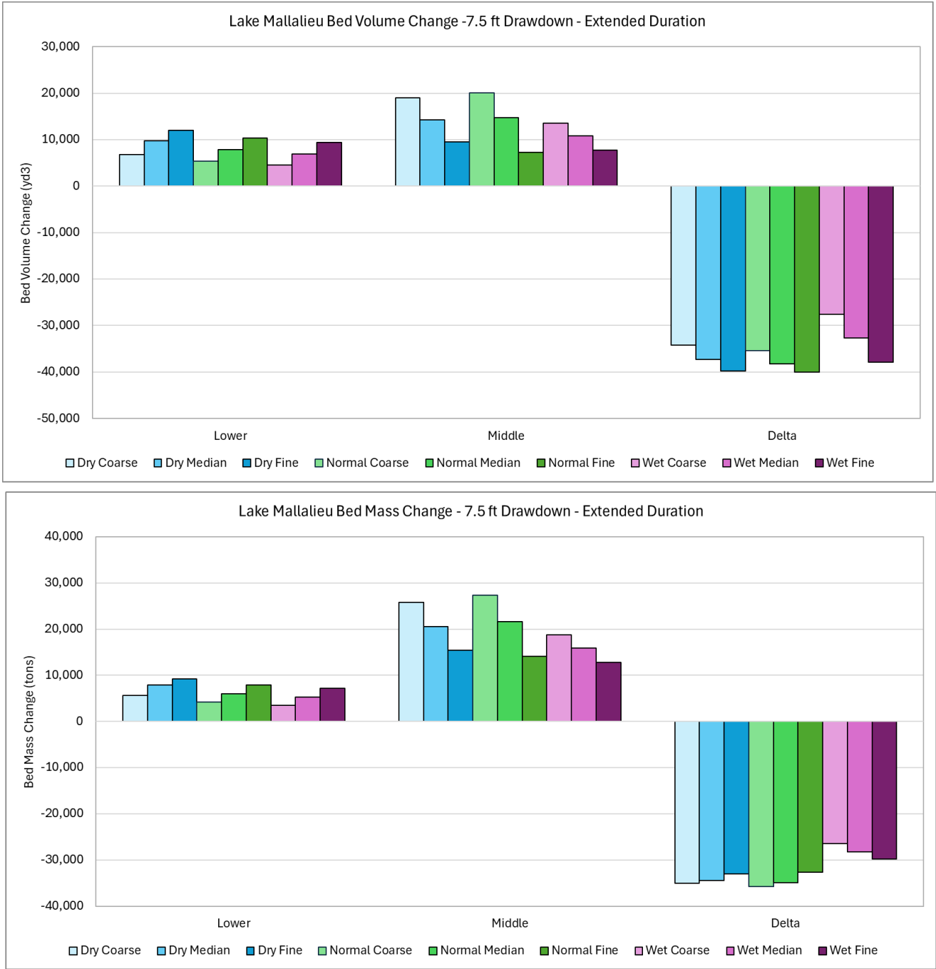
Figure 18. Changes in bed volume (top) and mass (bottom) for segments through the Lake Mallalieu impoundment during the extended drawdown period of September to July for the 7.5 ft drawdown.
