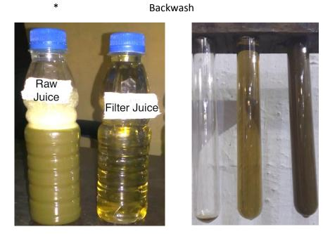
Sugar clarification trial with KERASIEV <sup>®</sup> Ceramic Membrane KERASIEV is a register trade mark of Need Inovation. Email: <u>mail@needinovation.com</u>,<u>needinovation@gmail.com</u> PH.0091 7980807924,9836467386, <u>www.needinovation.com</u>
