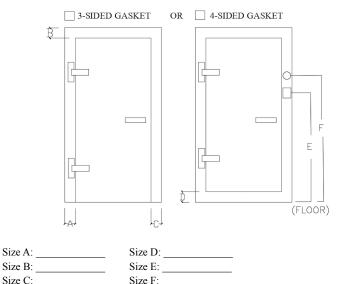
**Note:** Coldrite standard face frame size is 6" on all sides. However, we can produce 4" minimum.
