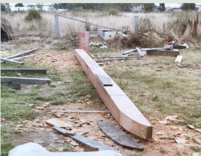
Her beginnings: a slab of wood (the keel) and a stack of timber (her planking) In the paddock on the hill, Ada St. Triabunna, 1979.
