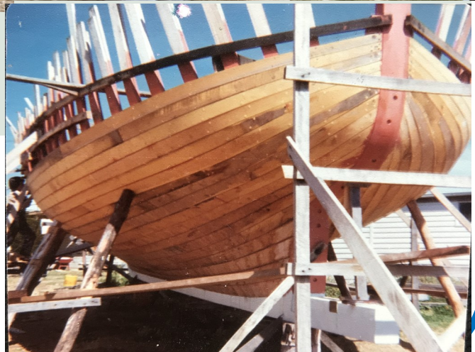
Her beginnings: a slab of wood (the keel) and a stack of timber (her planking) In the paddock on the hill, Ada St. Triabunna, 1979.
