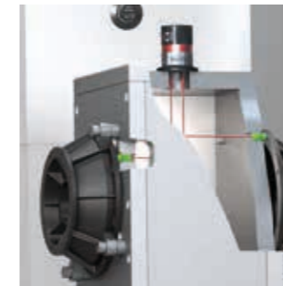
TG81 – with up to 8 sensors in the workpiece clamp fixture
