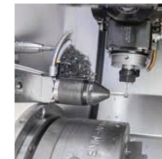
Tool measurement – TC76 with protective sleeve
