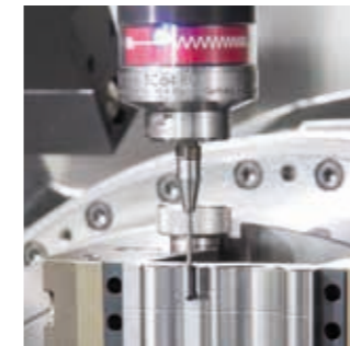
TC64-RG – Roughness measurement in the machining centre
