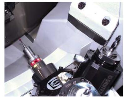
Fast workpiece measurement in rotary transfer machine
