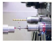
Workpiece measurement on turning machine
