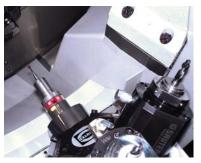
Fast workpiece measurement in rotary transfer machine
