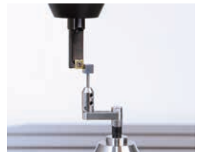
Tool radius measurement with special probe configuration
