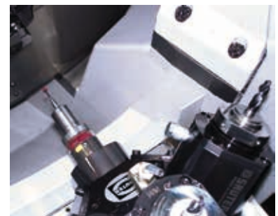
Fast workpiece measurement in rotary transfer machine
