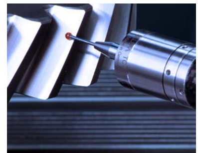
Workpiece measurement in grinding centre
