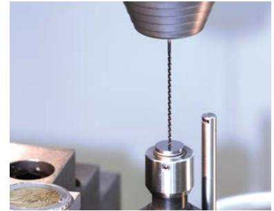
Fast tool breakage detection
