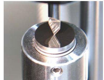
Extremely low measuring force enables the measurement of most sensitive tools
