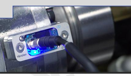
DTect-IT is a Windows application that communicates with custom Caron Engineering USB sensors to effectively monitor any area of concern on your CNC machine tool or fixture. Using sensors for *vibration, strain, high-precision power,* and *analog,* the user can establish a baseline of characteristics to determine when irregularities are present.
