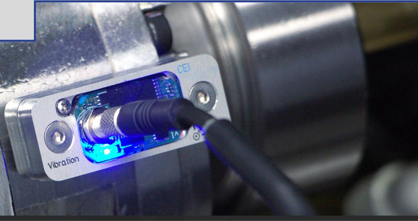
D-Tect-IT is a Windows application that communicates with custom Caron Engineering USB sensors to effectively monitor any area of concern on your CNC machine tool or fixture. Using sensors for **vibration, strain, high-precision power, and analog**, the user can establish a baseline of characteristics to determine when irregularities are present.
