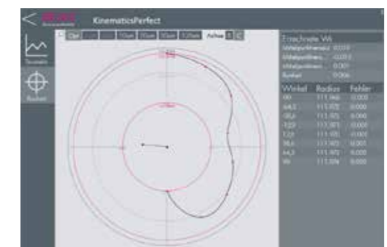
Displays evaluation of circular deviation, centre drift and individual measurements of the C-axis
