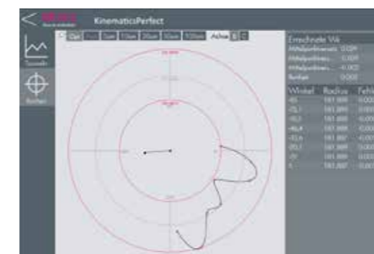
Displays evaluation of circular deviation, centre drift and individual measurements of the B-axis
