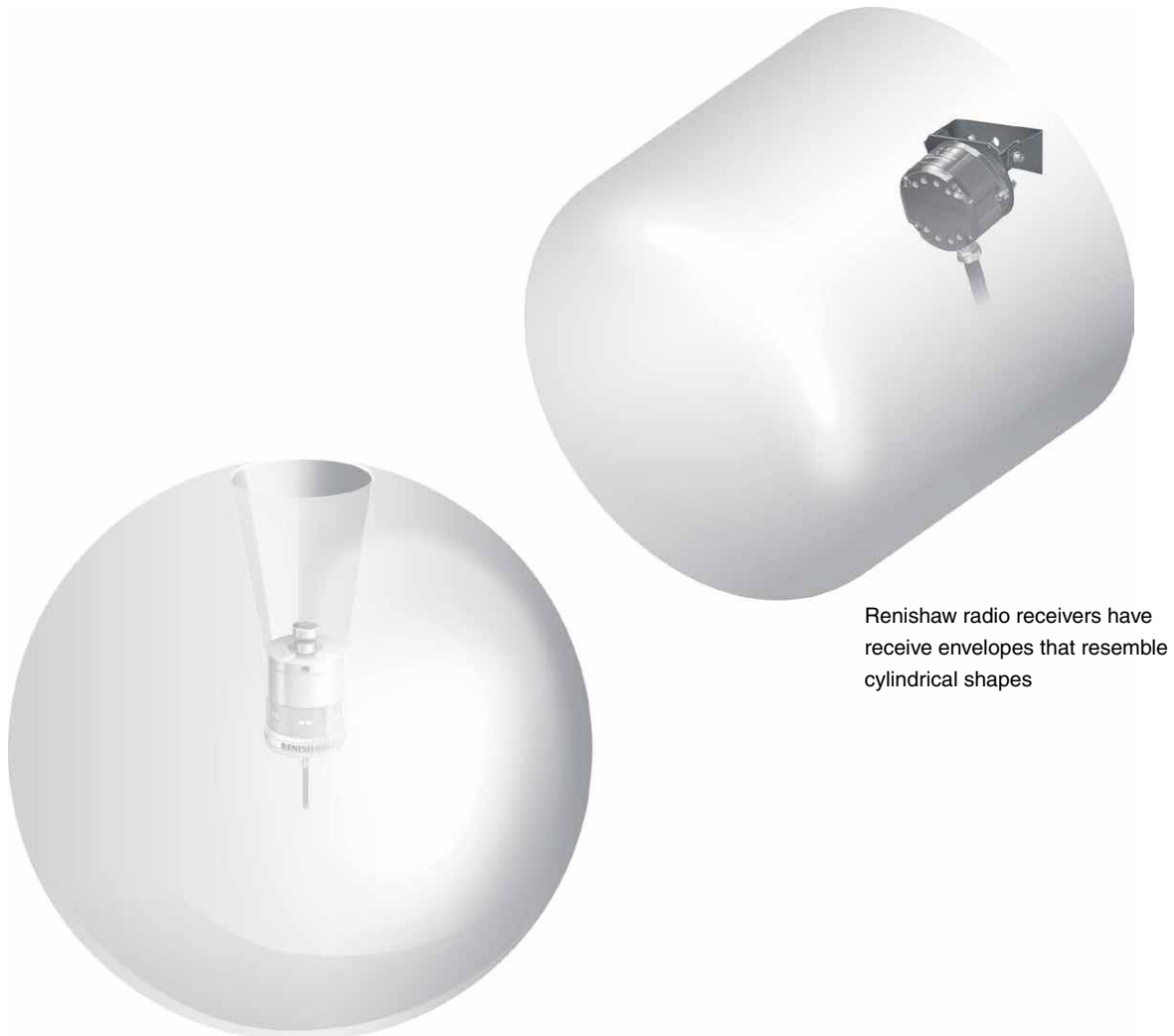
Renishaw workpiece probes have transmission envelopes that resemble spherical shapes
