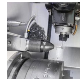
Tool measurement – TC76 with protective sleeve
