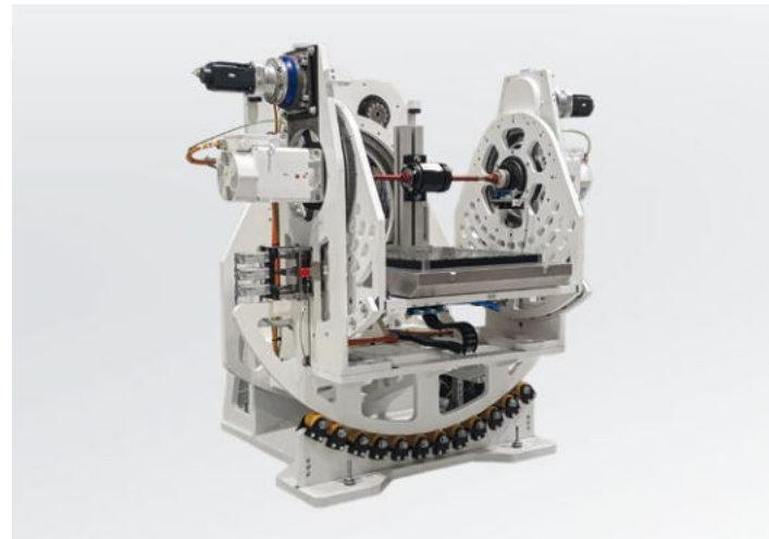
Swivel test bench for E-Drive and AWD products
