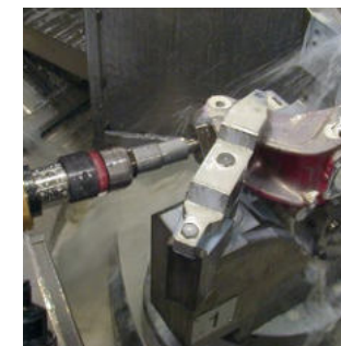
Measurement of a steering knuckle bore before slitting
