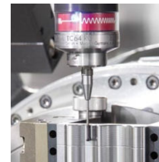
TC64-RG – Roughness measurement in the machining centre
