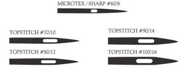
In 1942 standard needle sizes were put in place and a metric size designation under the abbreviation Nm (Number Metric) was introduced. It indicates the diameter of the needle blade in hundredths of a millimeter measured above the scarf. For example, an Nm 90 needle is .9 millimeter in diameter, while a Nm 60 needle is .6 millimeter in diameter.
