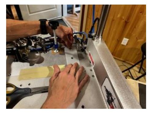
Peel the backing off the front section of the Grip that will go under the clamp bar and cut off backing.
