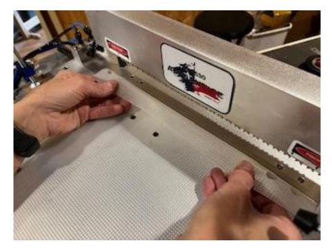
Remove the masking tape and peel the remaining backing off the grip.
